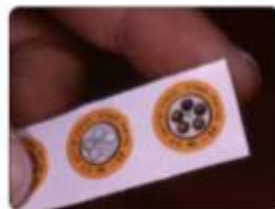
ColorCheck with 5 temperature levels. ColorCheck are also available with other temperature values and temperatures.
