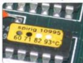
ColorCheck with 5 temperature levels. ColorCheck are also available with other temperature values and temperatures.
