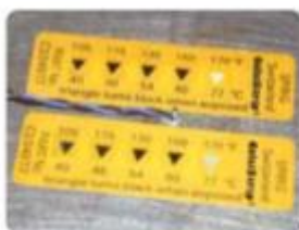
ColorChange with 5 temperature levels. Also 6 levels (see above) are available. Max 60°C are recorded for TTC never marked.
