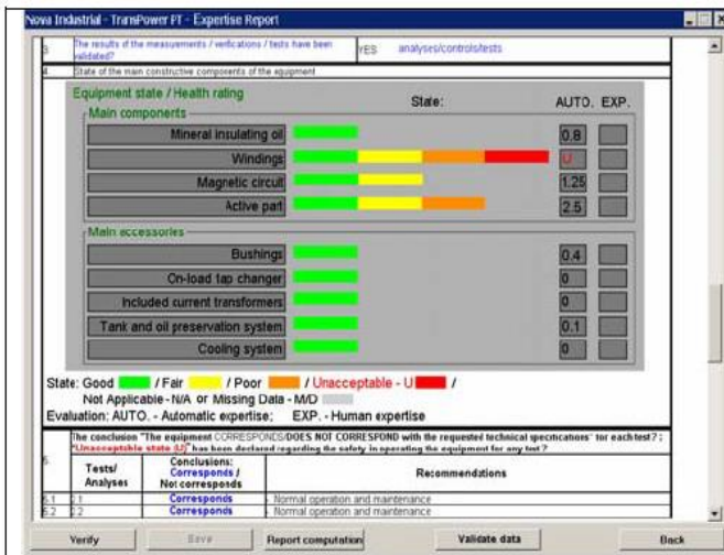
a - Display of condition indicators for an 200/200/60 MVA 231/121/10.5 kV autotransformer - TRANSPower - PT module
