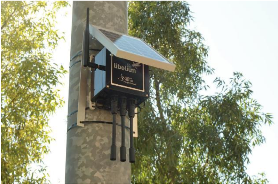
Figure 19: A Wasp mote sensor-node by Libelium, can be easily installed in a light pole (source: http://www.libelium.com/products/plug-sense/technical-overview/ )
