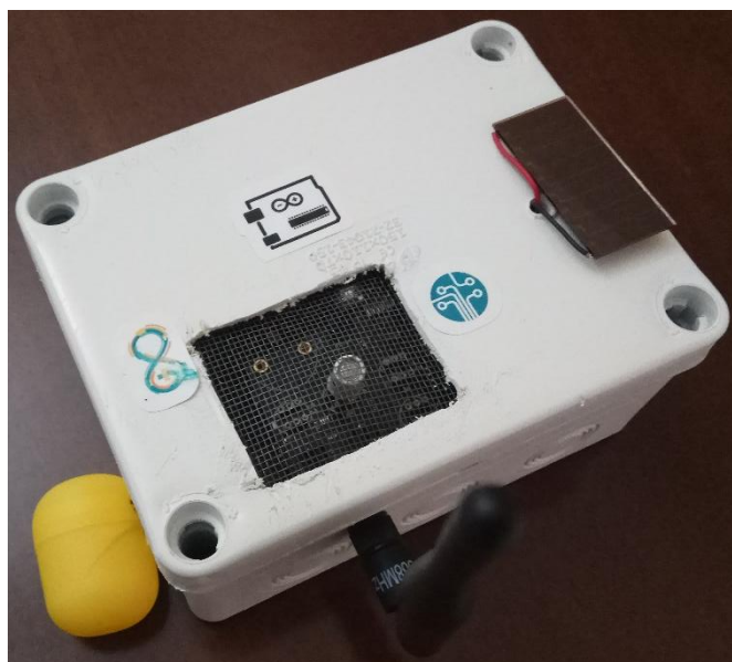
Figure 24: Top-side view of the node. The dust filter enables the sensors to have exposure to the environment.
