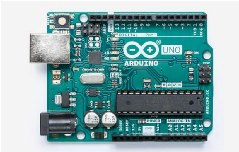
Figure 4: The Arduino UNO development board. Its pin layout has now become a standard and it is used by many other companies (source: https://store.arduino.cc/usa/arduino-uno-rev3 )
