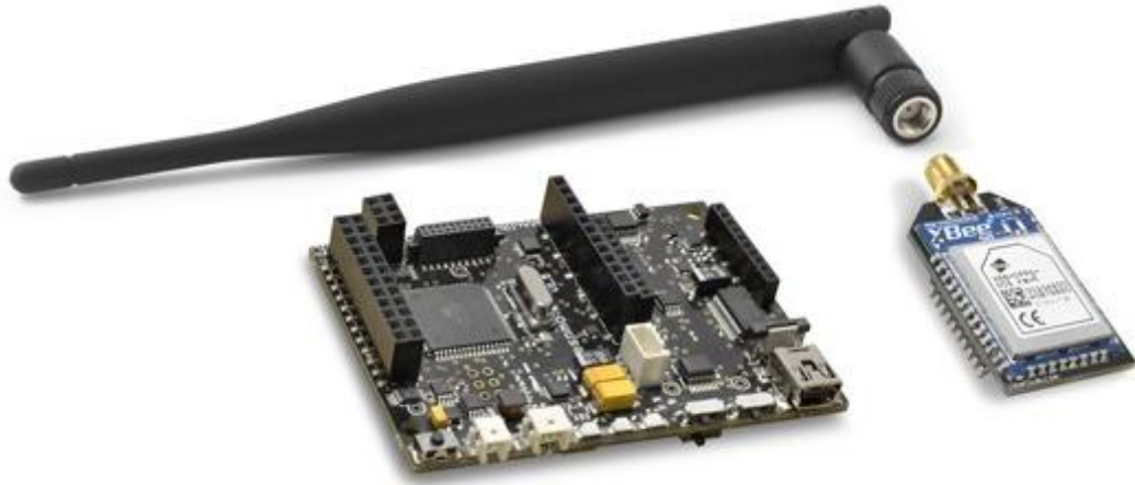
Figure 23: The Wasp mote (left), the XBee module (right) and its antenna (top) (source: https://www.cooking-hacks.com/Waspote-868-sma-4-5-dbi )
