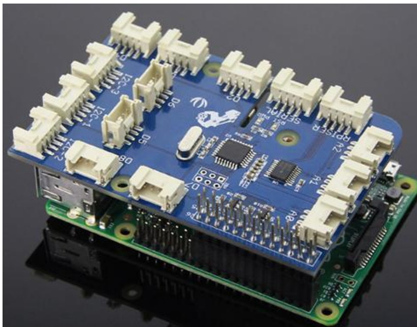
Figure 20: The GroovePi+ HAT embedded on top of a Raspberry Pi SBC. The HAT provides an interface for connecting Grove sensors to the Pi (source: http://wiki.seeedstudio.com/GrovePi_Plus/ )
