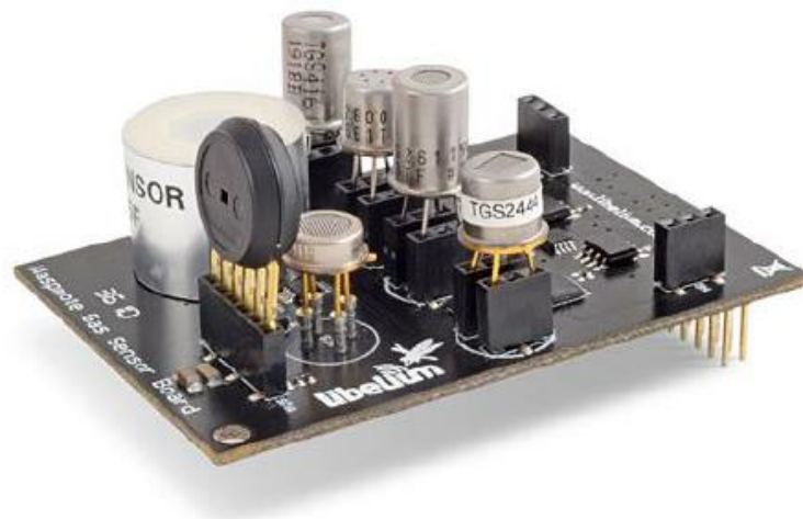
Figure 6: The shield for the Waspote that is used for air-quality and gases monitoring, alongside the sensors (Waspote gases sensor board, source https://www.cooking-hacks.com/Waspote-gasses-sensor-board )
